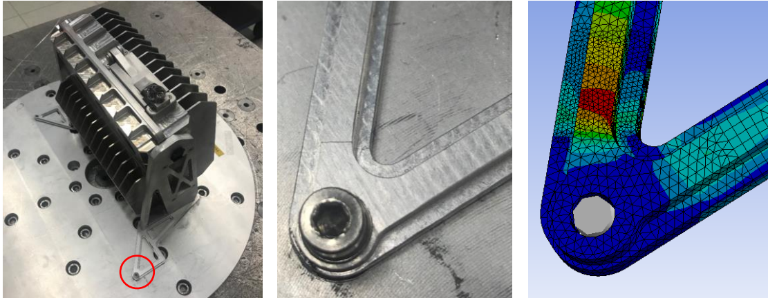
Figure 7.17 Observed crack in 48 minutes
