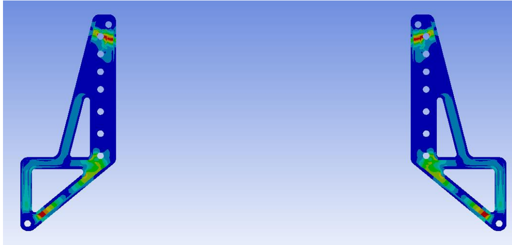
Figure 4.11 High stress regions of the structure except for singularity areas
