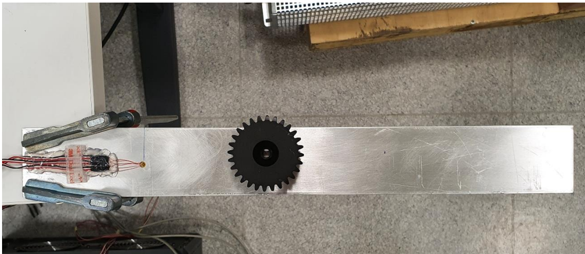
Figure 3.2.3 Strain Gauge Verification Test Set-Up for Distance 100 mm
