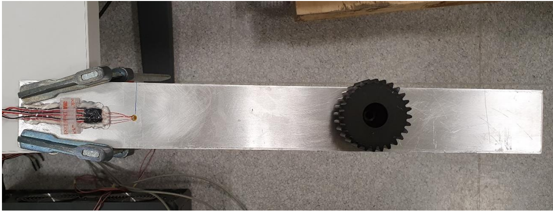
Figure 3.2.2 Strain Gauge Verification Test Set-Up for Distance 200 mm
