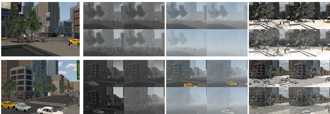
FIGURE 4.7.: The figure demonstrates the weather variations simulated in PTAW217Synth. The first and second rows present different view points of the same location. Each group of 2x2 images shows one weather condition (from left to right: rainy, foggy, and snowy) in increasing adversity while the leftmost image shows the same location in clear weather.
