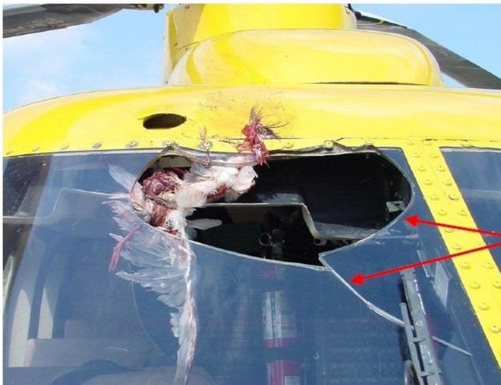
Figure 2-5 Bird Strike on Sikorsky S-76A++ with the STC Acrylic Windshield [13]
