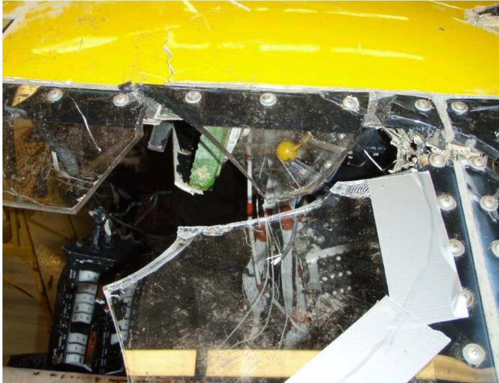
Figure 2-4 Reconstruction of the Sikorsky S-76A++ Canopy and Windshield [13]
