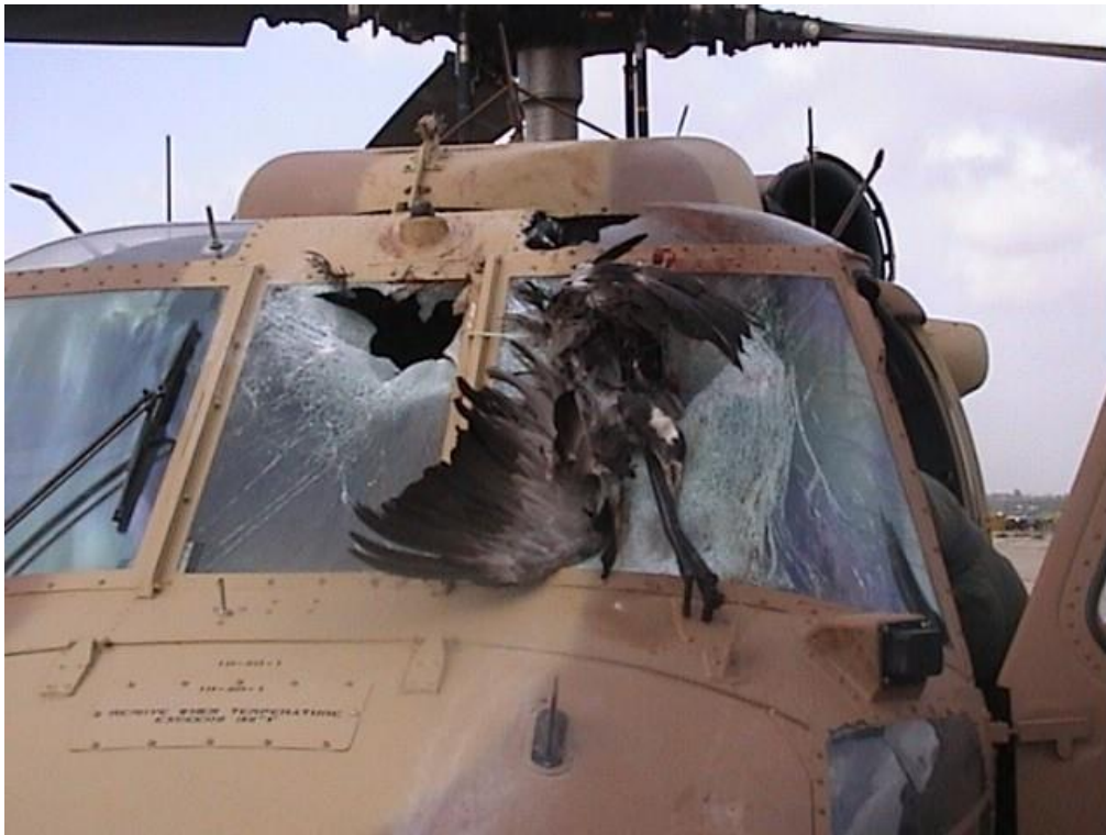
Figure 2-1 Sikorsky UH-60 Helicopter after Birds Strike, Outside
