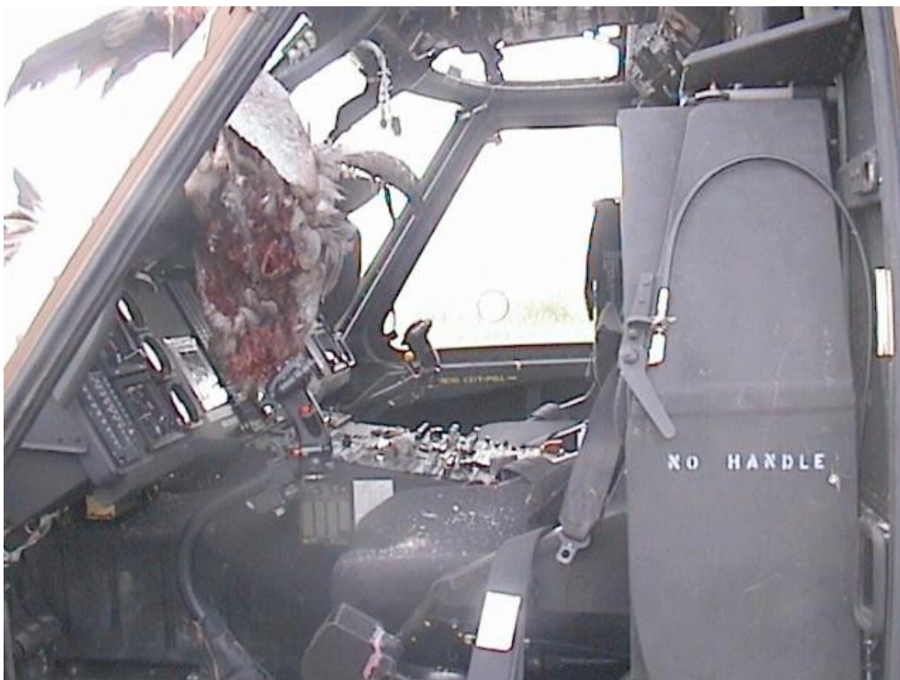
Figure 2-2 Sikorsky UH-60 Helicopter after Birds Strike, Inside
