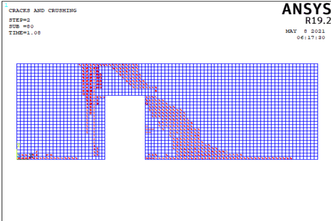
Figure 5.14. The Crack Pattern of Wall 1 Model 11 According to Compressive Strength Values of (a) 3 MPa, (b) 8 MPa
