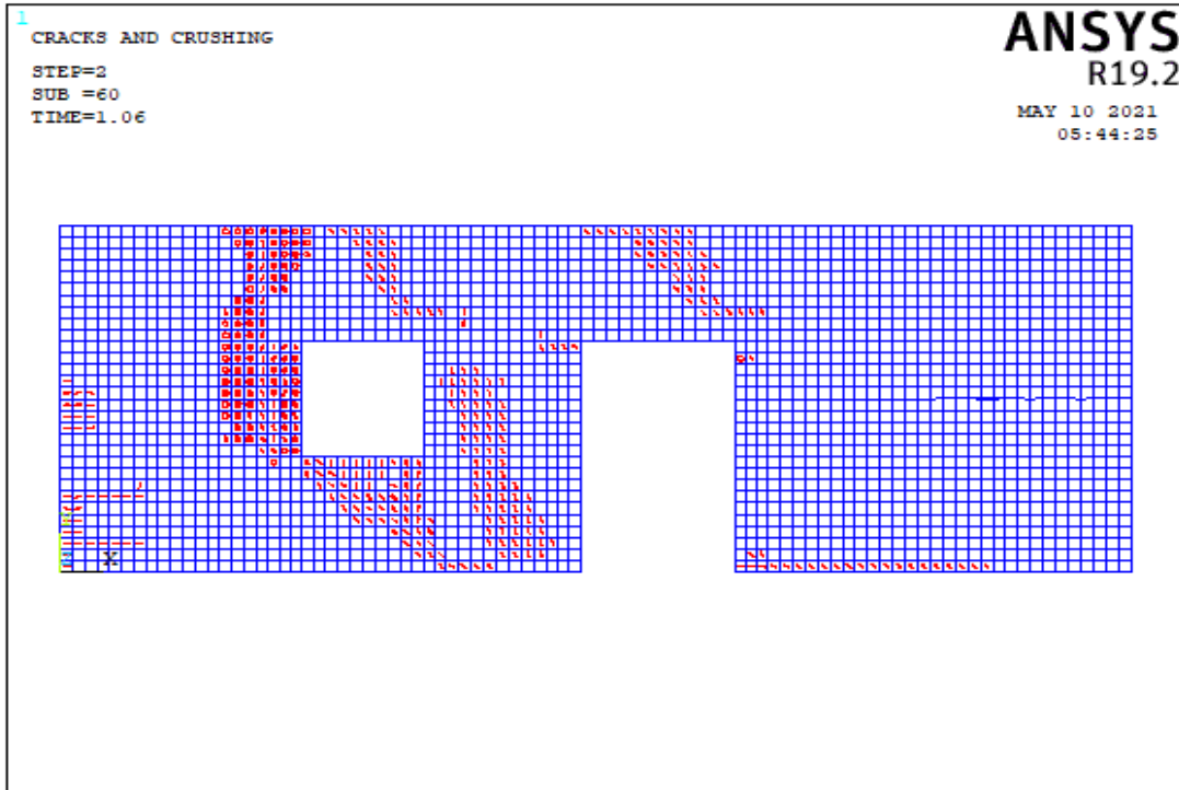
Figure 5.102. The Crack Pattern of Wall 12 Model 7 According to Compressive Strength Values of (a) 3 MPa, (b) 8 MPa
