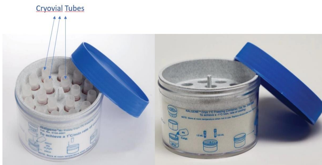
Figure 3.8. Mr. Frosty™ Freezing Container adapted from Thermo Scientific (156). (147)
