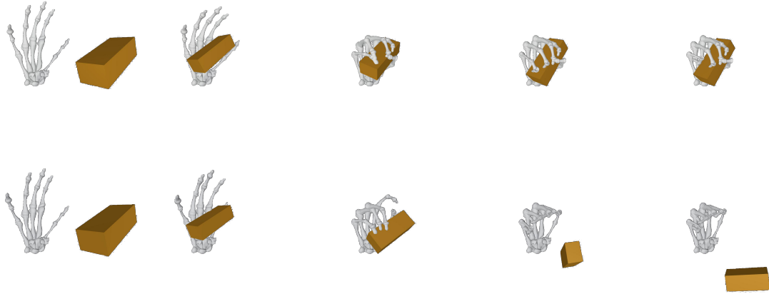
Figure 6.8: The comparison of trained proactive brain (up) and heuristic proactive brain (down) for catching a rectangular prism with skeleton hand model.
