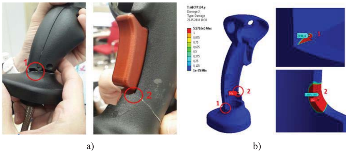
Figure 3-32: The damaged part: a) Test result; b) FEA result
