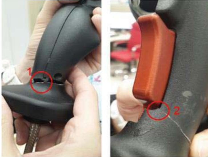
Figure 1-2: The control column damaged by accelerated tracked vehicle vibration testing
