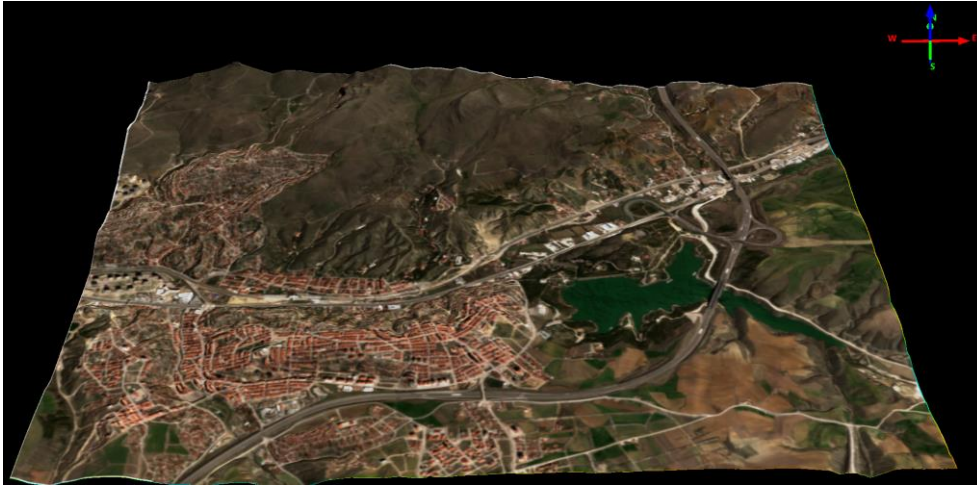
Figure 6.4. The digital terrain model that has a textured surface with the Sentinel-2 image.
