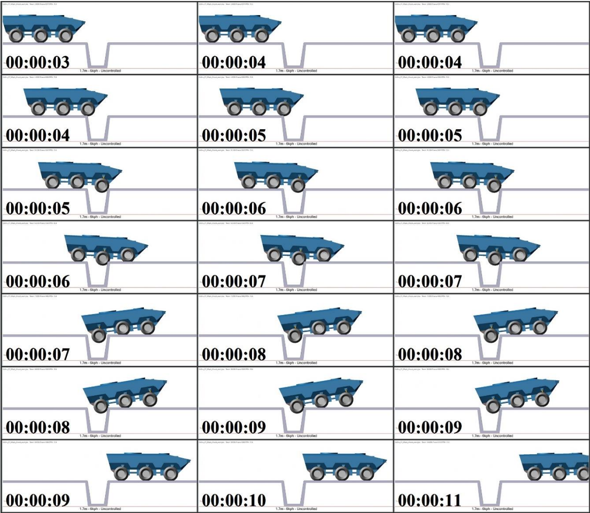
Figure 5.30 Trench crossing 1.7 m, 6 kph, uncontrolled
