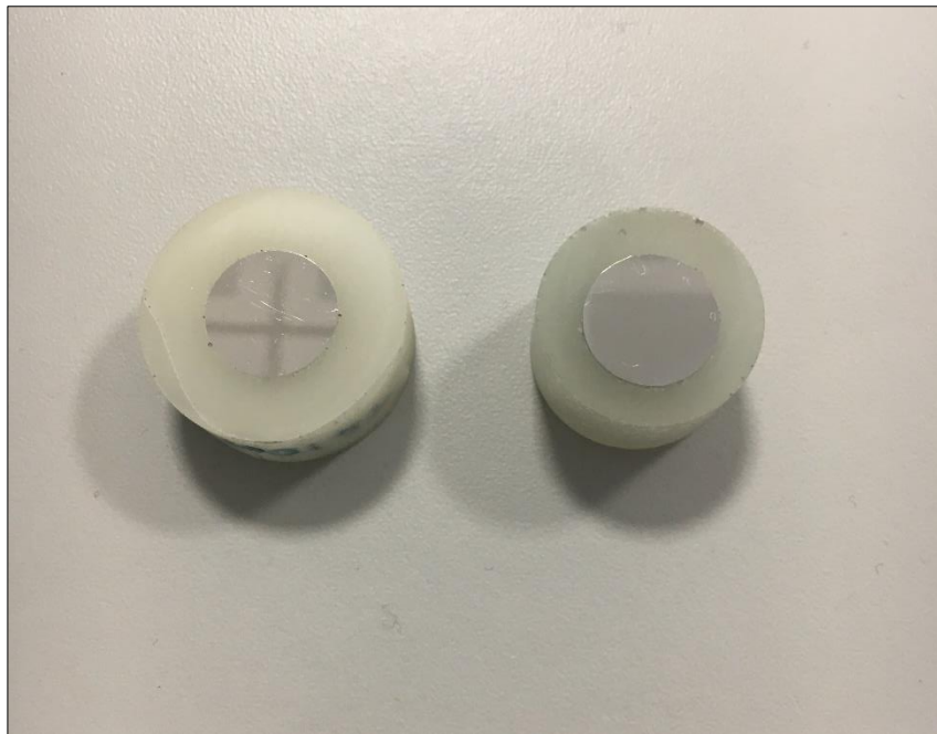
Figure 3-2: Polished faces of the specimens.
