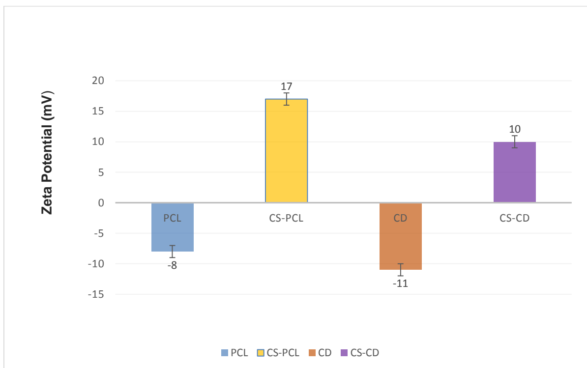
Figure 4.9. Zeta Potential values of CPT loaded PCL, CS-PCL, CD and CS-CD nanocapsules. Data represents the mean results \pm SD values of three different batches.
