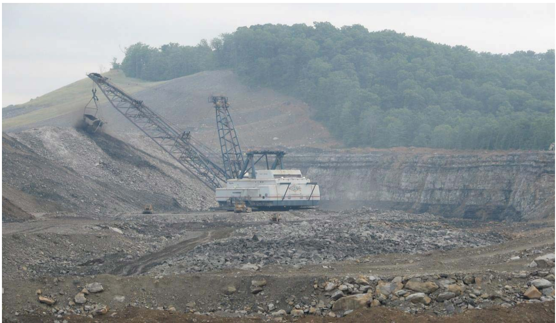
Fig. 2. A Dragline. Courtesy of the photographer, Vivian Stockman from the Ohio Valley Environmental Coalition.
