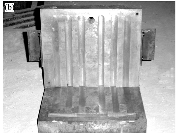
Fig. 2: (a) Schematics of fluidity test mold, and (b) image of corresponding mold
