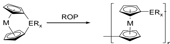
Scheme 2. Ring Opening Polymerization of an ansa Metallocene
