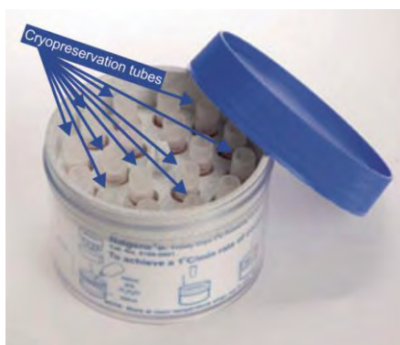
Figure 3.12. Nalgene Mr. Frosty achieves a rate of cooling close to -1^{\circ}\text{C} per minute. Adapted from Thermo Scientific (227).
