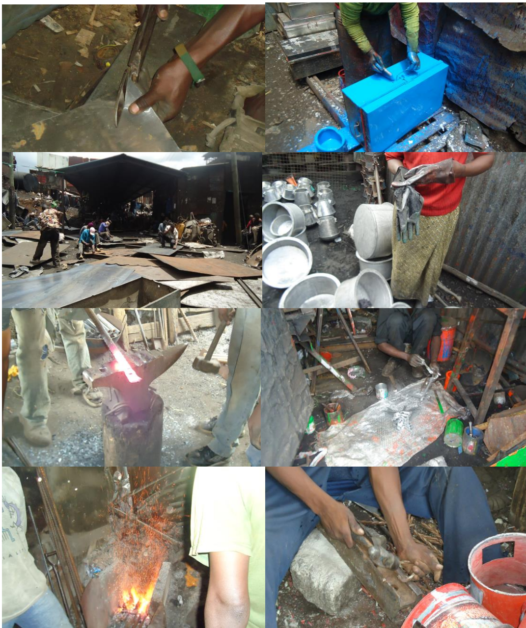
Activities carried out in Kamukunji Jua Kali (from top left): cutting metal sheet; painting; cutting and folding of metal sheets; pickling of the final products; heat treatment, moulding, folding and cutting; aluminium coating; heat treatment, and folding metal rods.
