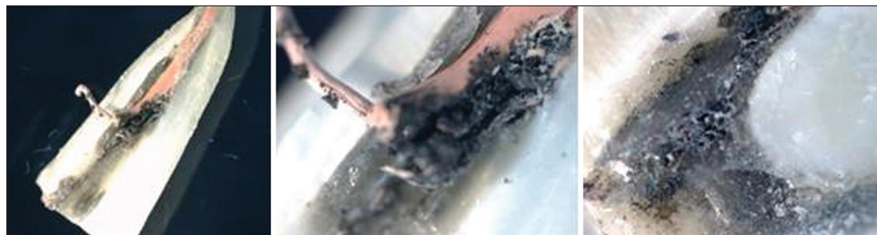
Figure 5: Stereomicroscope views: 50 mJ/pulse laser: Remaining gutta-percha and some carbonized parts were observed
