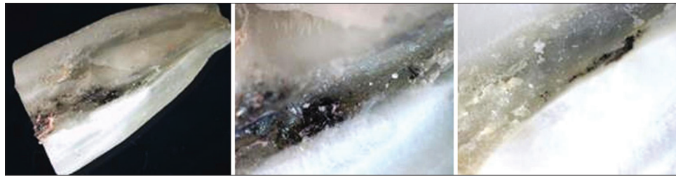
Figure 7: Stereomicroscope views: 50 mJ/pulse laser: Carbonization was observed in <50 mJ/pulse laser and in 135 mJ/pulse laser (control group)
