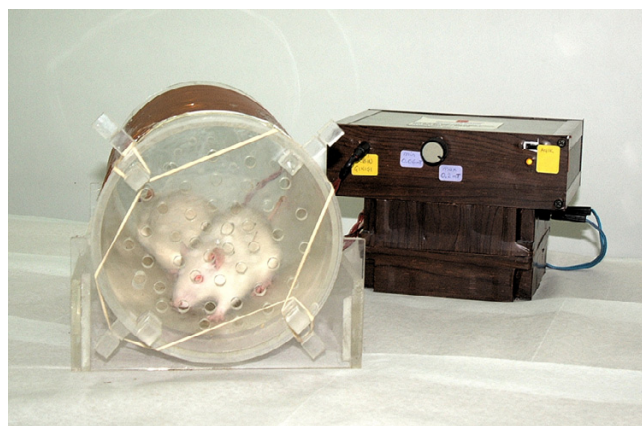
Figure 1 Fabricated custom-made device to deliver PEMF stimulation on osteoporotic rats.
