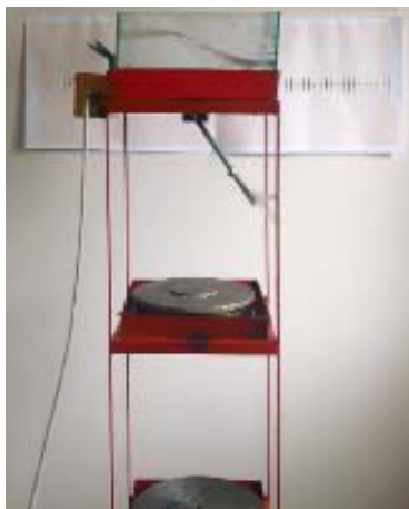
Fig. 4. 3-storey Building shear frame model with TLD
