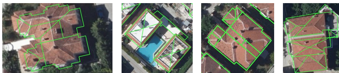
Figure 20. Examples to the false reconstructions of the roofs.
