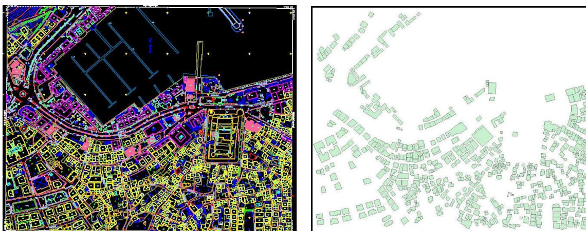
Figure 7. A part of the basemap with all CAD layers (left) and the building footprints extracted from a set of them (right).
