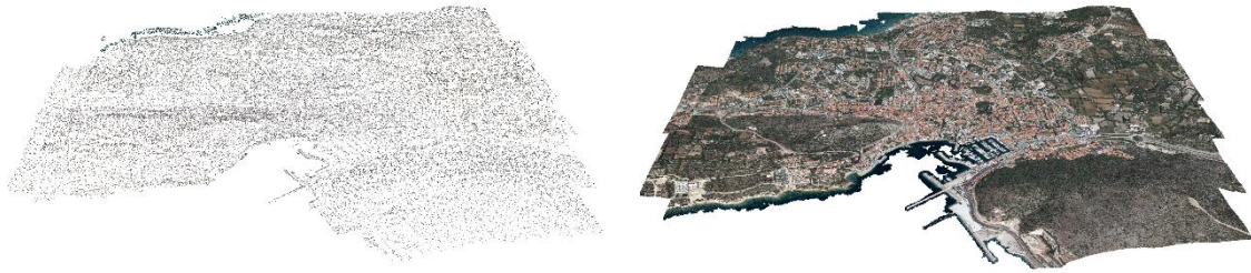
Figure 10. Generated tie points (left) and dense point cloud (right) using Agisoft Photoscan.
