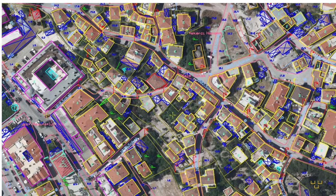
Figure 6. Manual feature extraction from stereo aerial images.
