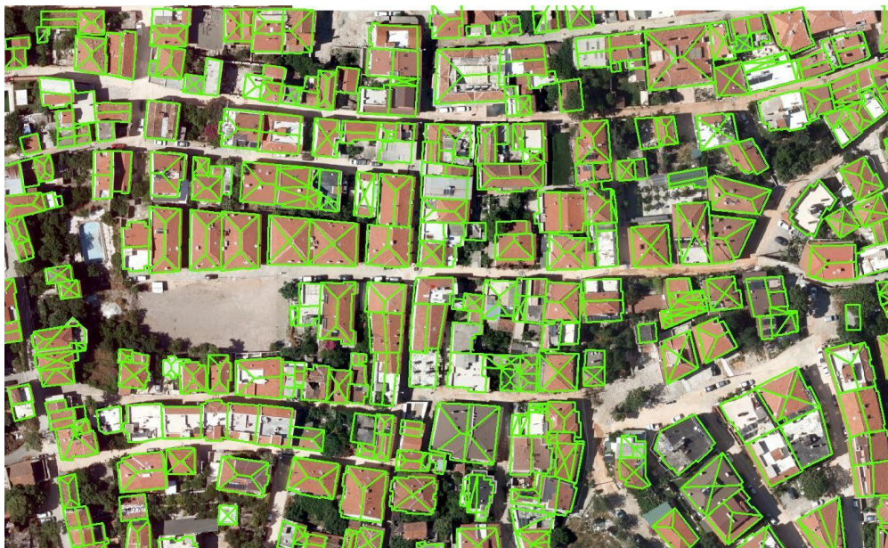
Figure 15. Automatically generated roof geometries overlaid on the orthophoto with 10 cm resolution.
