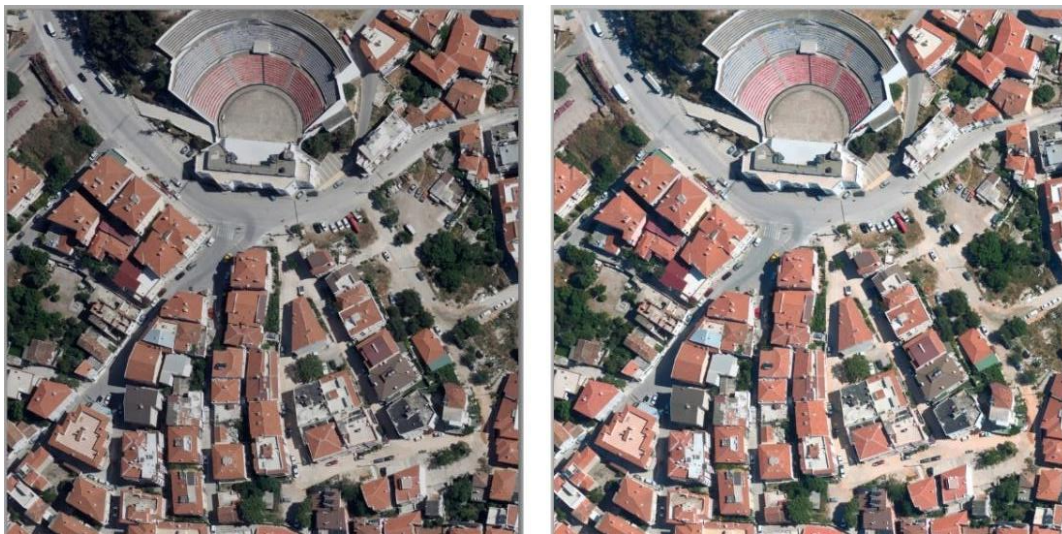
Figure 17. Raw aerial image (left) and pre-processed (color-enhanced) image (right) of Cesme Town.
