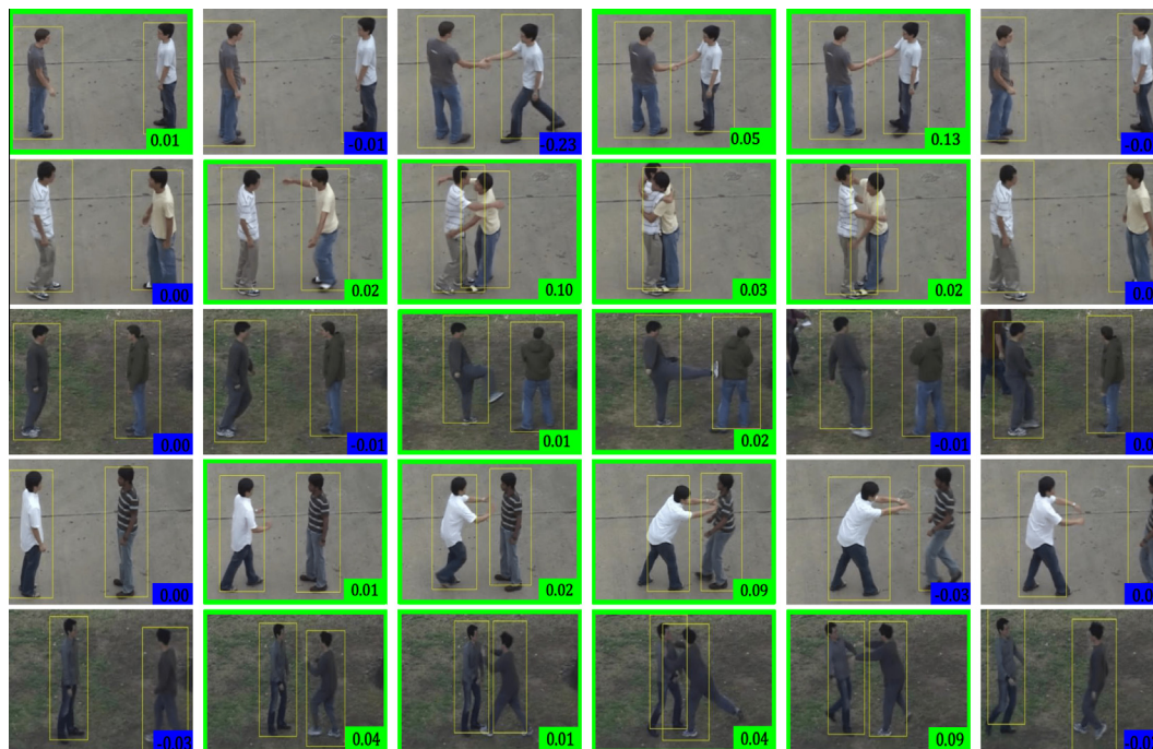
Fig. 5. The contributions of individual frames to the classification using our approach on UT-Interactions dataset [40]. In this figure, from top to bottom, the videos belong to hand shake, hug, kick, punch and push classes, from SET1 and SET2 divisions of the dataset. The yellow bounding boxes show the person tracks that are acquired automatically via person detection and meanshift tracking. The contribution scores are displayed on the bottom right corner of each frame and the instances with positive contribution scores for each target interaction are marked with green. As it can be observed, while there are some confusions, overall, our algorithm is quite successful in discriminating the frames related to each interaction. (For interpretation of the references to color in this figure legend, the reader is referred to the web version of this article.)
