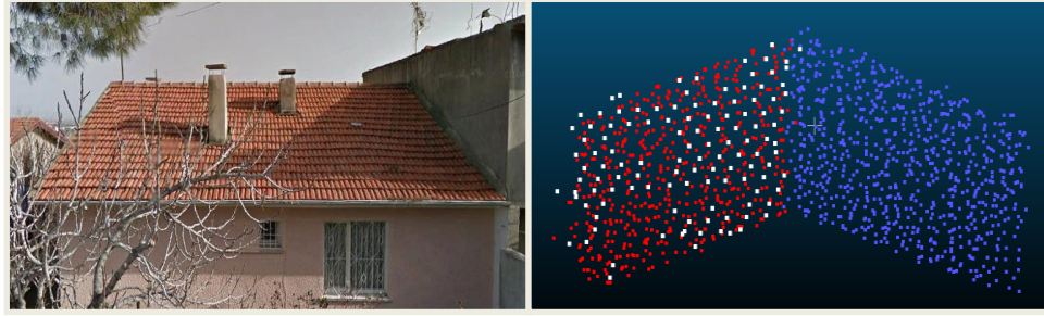
Figure 4.25. A, building (Building #10) with the extracted parallel planes (the plane of white data points and the plane of red data points).
