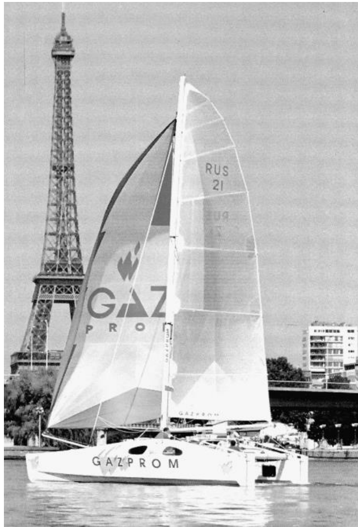
Figure 2.2. Ivan-30 (Catamaran yacht) made from carbon-epoxy composite [3].
