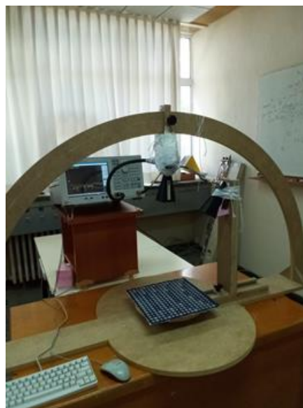
Figure 6.8. Measurement setup for offset feed configuration.
