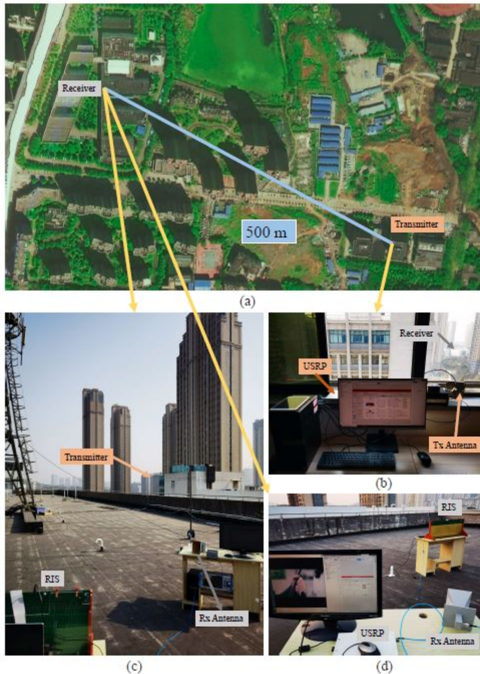
Figure 2.16 Outdoor measurements for the IRS at 5.8 GHz [10].
