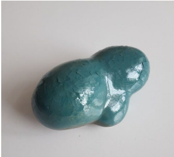
Figure 51. Test piece painted with copper solution, with a shiny, cracked finish.
