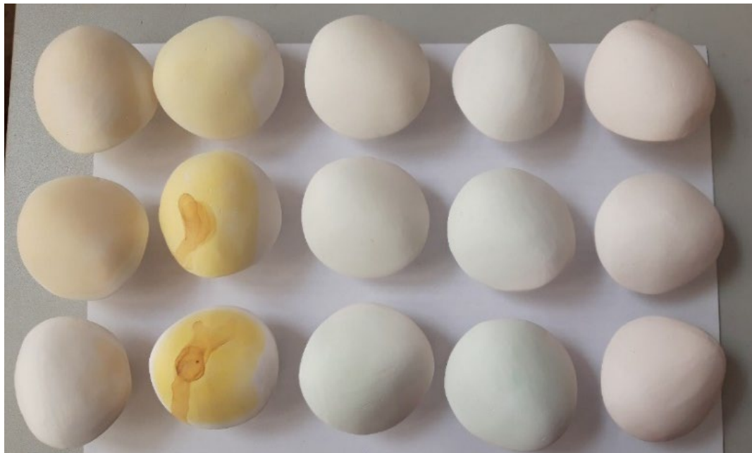
Figure 46. From left to right: Iron Sulfate, Iron III Chloride, Nickel Sulfate, Copper Sulfate and Cobalt Sulfate. From top to bottom: low percentage to high percentage solutions.
