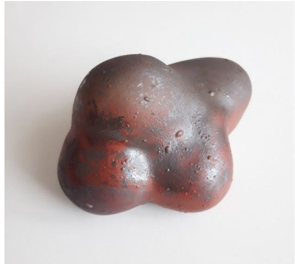
Figure 52. Test piece painted with iron solution, with a metallic, rust like finish.
