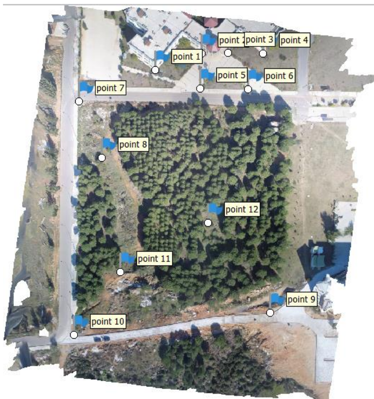
Figure 4.3: UAV orthorectification with GCPs
