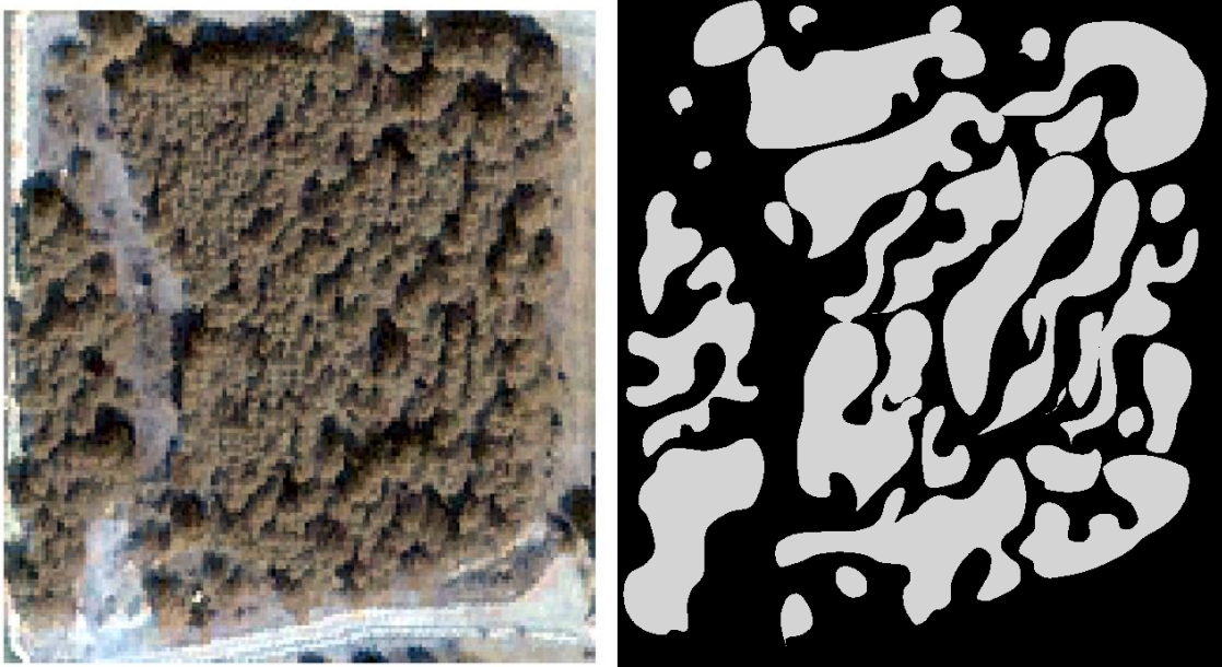
Figure 3.10: GK-1 MS image (left) and the manually delineated ground-truth map (right) part in the study area.
