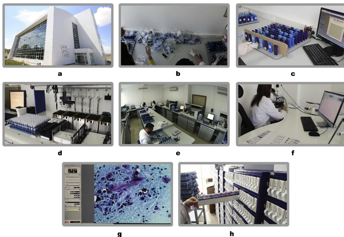
Fig. 1. Flowchart of the National HPV Laboratory. 1a National HPV Lab is on Floor 2 with 7 Rooms, 1b Two barcoded sample from the same patient (conventional cytology and HPV DNA) arrives to the laboratory by Cargo, 1c Barcoding system and software does not allow any mismatch among the millions of samples received 1d Rapid Capture System (RCS) by Qiagen ® 1e 10 RCS System works simultaneously to detect HPV DNA 1f -1g Cyto-pathologists evaluating the pap Smears in a double blind manner and saving the digital pictures (cyto-gallery) 1h Storage of the positive (5 Years) and negative samples (3 months).
