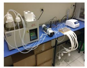
Figure 1. Drip flow reactor used in the study
