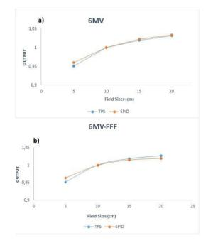
Figure 1. The measured and calculated output factor comparison between iViewDose and beam data commissioning
