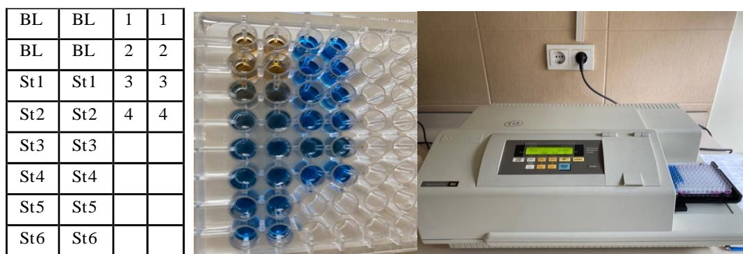
Figure 3.8. Determination of protein concentration. For the determination of protein concentration 96 well plate was loaded as shown in the template and after addition of the reactive (Bio-Rad Cat No: 5000 006), the absorbance of the wells were measured by a microplate reader (Molecular Devices Spectramax M2, USA) and the protein concentration of the samples were calculated according to the standards. BL: Blank, Standard 1 (St1)-Standard 6 (St6): 12,5-75 \mu\text{g/ml} BSA. Lysates of DPSC incubated for 21 days in 1 ; Growth medium ( GM ), 2 ; growth medium+Melatonin (10 \mu\text{M} ) ( GM+MT ), 3 ; dopaminergic neuronal differentiation medium ( DNM ), 4 ; dopaminergic neuronal differentiation medium+Melatonin (10 \mu\text{M} ) ( DNM+MT ).
