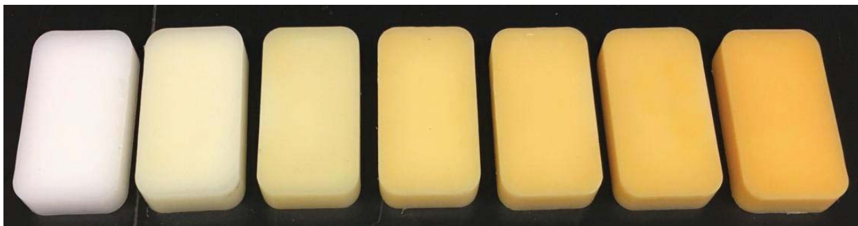
Figure 8. 8. The display of UHMWPE/GS with various concentrations. From left to right; virgin UHMWPE, 1, 2, 4, 6, 8 and 10 % GS.
