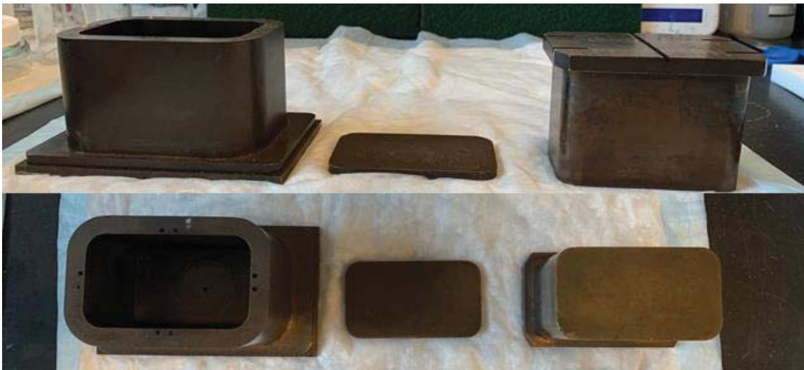
Figure 7. 3. Components of the aluminum-bronze alloy mold; mold (left), insert plate (middle), plunger (right).
