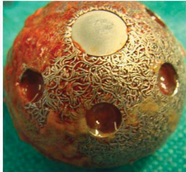
Figure 3. 1. Biofilm related failure of titanium hip acetabular implant (Lentino 2003).
