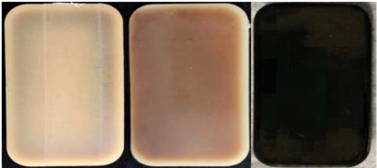
Figure 8. 2. Color change of UHMWPE loaded with 8 wt. % gentamicin sulfate molded at 170 °C for 8 min (left), 20 min (middle) and 2 hour (right)
