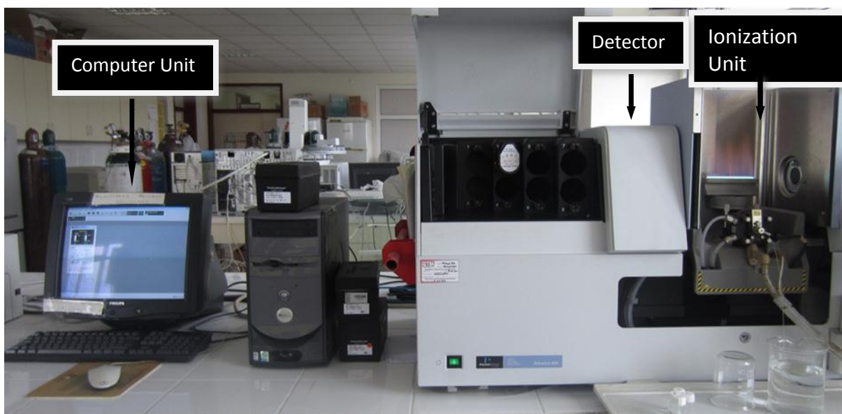
Figure 3.5. Atomic absorption spectroscopy instrument.
