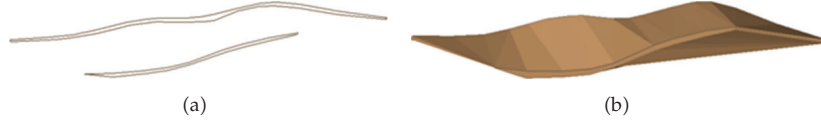
Figure 5: Nonplanar sections (a) and their three-dimensional models (b) which are used in 3D orebody modelling.
