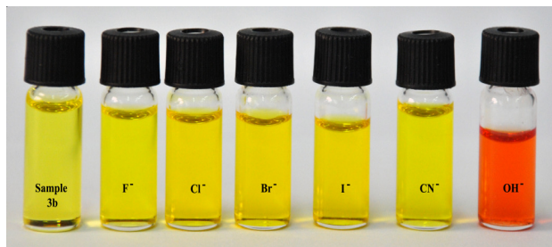
Fig. 4. Changes in the colour of 5 \times 10^{-5} M DMSO solution of receptor 3b . From left to right, in the absence of ions, in the presence of 1 equiv. of tetrabutyl-ammonium anions; fluoride, chloride, bromide, iodide, cyanide and hydroxide
