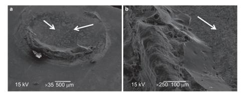
Figures 4 Representative SEM image of MIXED2 type of failure (cohesive failure of the veneering ceramic with >1/3 left adhered on the framework material). (a) Magnification ×35; (b) magnification ×250. Note the remnants of the veneering material on the zirconia substrate indicated by arrows. SEM, scanning electron microscope.
