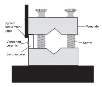
Figure 2 Schematic drawing of the fixation device where the ceramic block was clamped.
