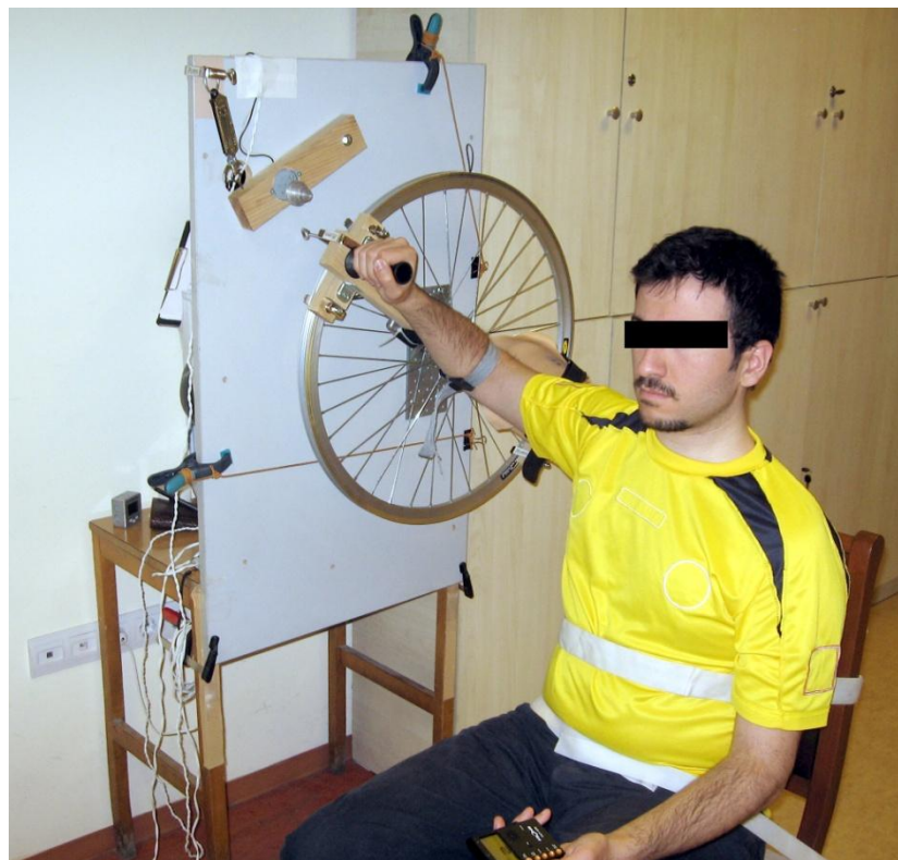
Figure 3.9. Adaptation of oPTD v2.0 for active movements through ROM at preset speed guided by metronome
